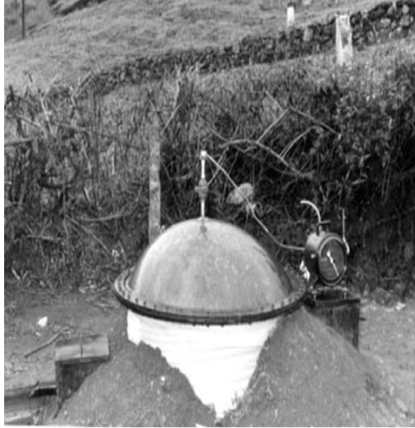
Figure 4: Localized (self-sufficient and contained) anaerobic methane digester 14
