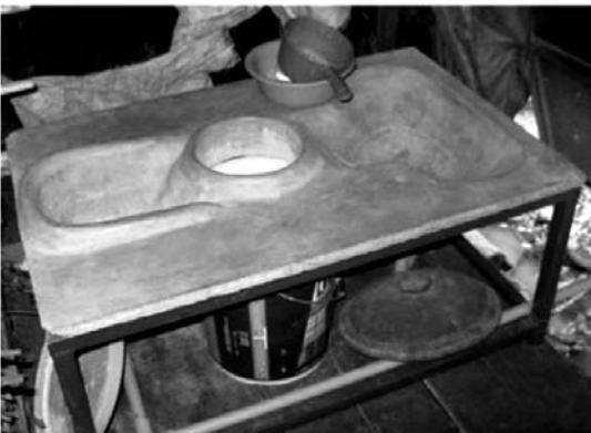
Figure 3: Locally made urination/defecation separation toilet (household scale) 13
