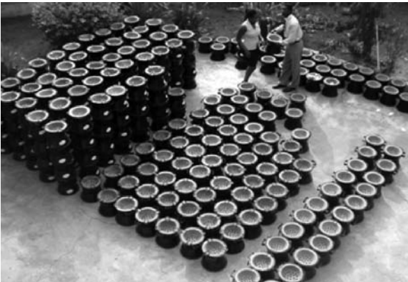
Production of Ceramic-Metal Jiko
